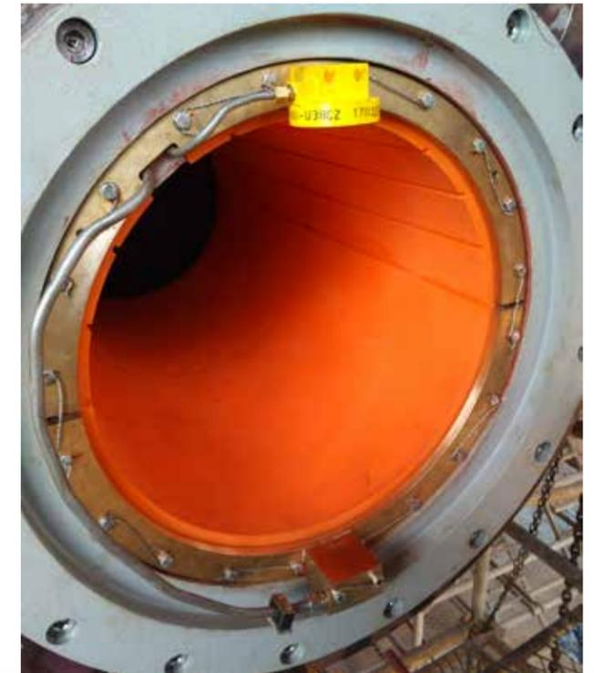
COMPAC propeller shaft bearing with Bearing Condition Monitor (BCM) System
