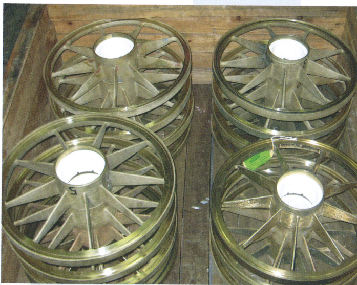
Thordon SXL pump bearings installed into existing bronze
