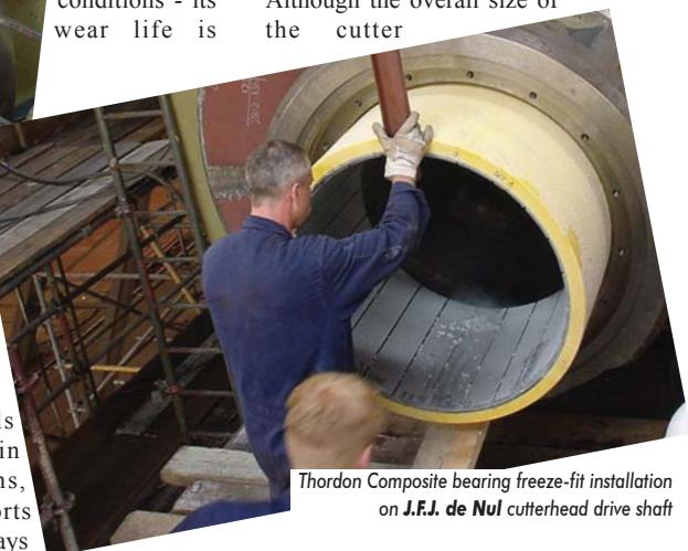
Thordon Composite bearing freeze-fit installation on *J.F.J. de Nul* cutterhead drive shaft
