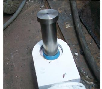
The ThorPlas-Blue SAB and hard coating pin system can be ordered in 4 standard pin sizes: 1.5", 2", 2.5", and 3", as well as in custom sizes.
